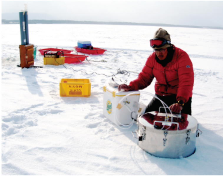
Figure 1. A picture showing the technique for measurements of the CO 2 flux by using a chamber technique at Saroma-ko lagoon, connecting to the Sea of Okhotsk, on the northern coast of Hokkaido, Japan.
