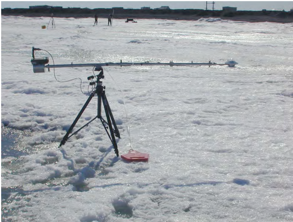
Kipp radiometer mounted on tripod.
