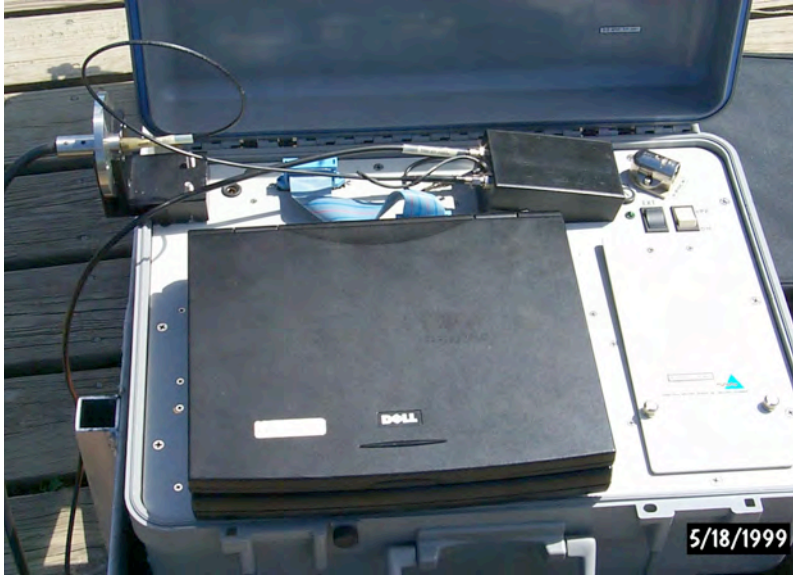
Gray box with computer mounted and fiber optics probes connected. Underice arm with cosine collected installed.
