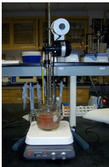
Figure 3. Picture of the laboratory apparatus to render oil from pollock liver
