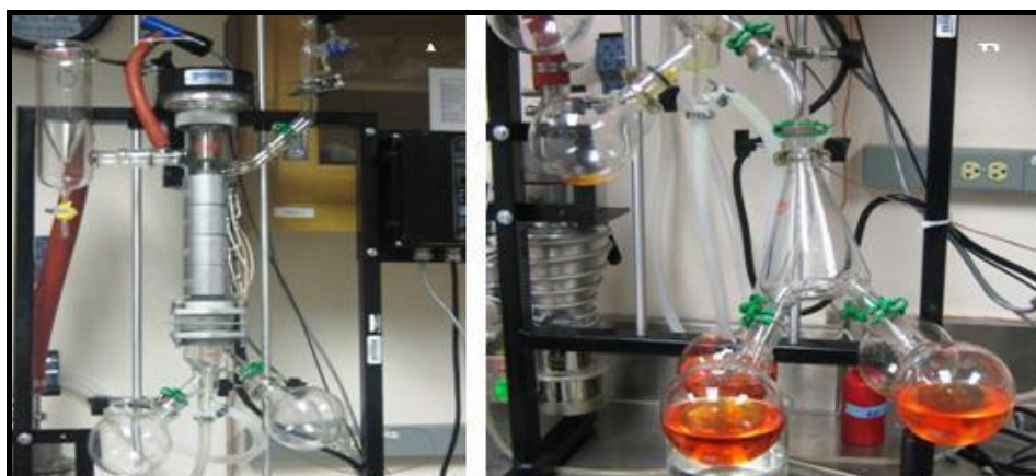
Figure 8. SPD system. (a) Evaporator showing exposed heating elements and fitted with one receiving flask and one residue flask; (b) Receiving flask glass joint adaptor ('cow') fitted with four receiving flasks
