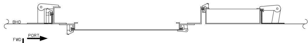
PLAN 7-A WET LAB DOOR AT FR 56 - LOOKING DOWN 1-1/2" = 1'-0"
